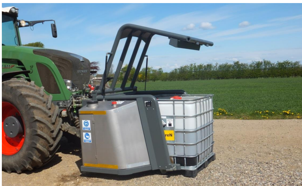
Fig. 9 Exchange of acid containers during acidification work at the field Source : Biocover Denmark 2015
