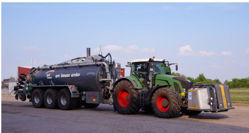
Fig. 7. Complete set driving to the field for providing spreading of acidification slurry Source: Biocover Denmark 2015
